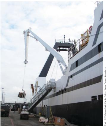
Shipboard pedestal cranes are used to move a wide range of materials safely and efficiently.
